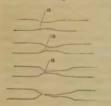
tube, a little above the thinnest part, but still not so much above as to render the thicker part the softest, let him carefully retract his right hand, by which operation the narrow part will become more and more attenuated, and finally, when capillary, fuse and separate. The end of the tube will be left closed of a
